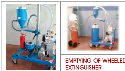
FILLING OF PORTABLE EXTINGUISHER
