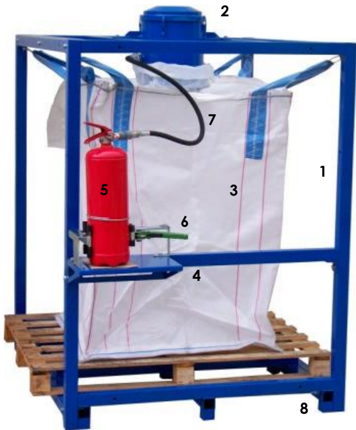
Powder recovery from a pressurized fire extinguisher
