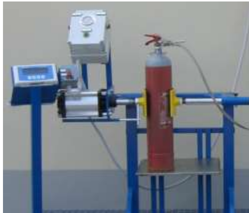
The AIR4-BIL clamps fire extinguishers during filling/recovery operations
