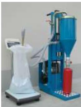
FILLING OF PORTABLE EXTINGUISHER WITH ETW100 SCALE
